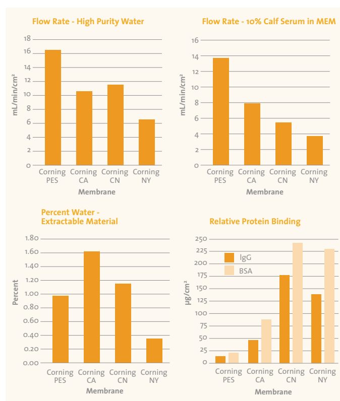
Figure 1. Important Performance Characteristics of Corning® Filter Membranes
